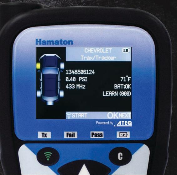
The tool will display the sensor's ID, battery status and frequency besides the tyre's pressure and temperature
